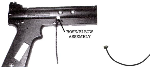
STEP 1. Remove plug from right side of marker know as the "Power Tube Plug" and Install HOSE ASSEMBLY by threading the universal fitting into the power tube.
